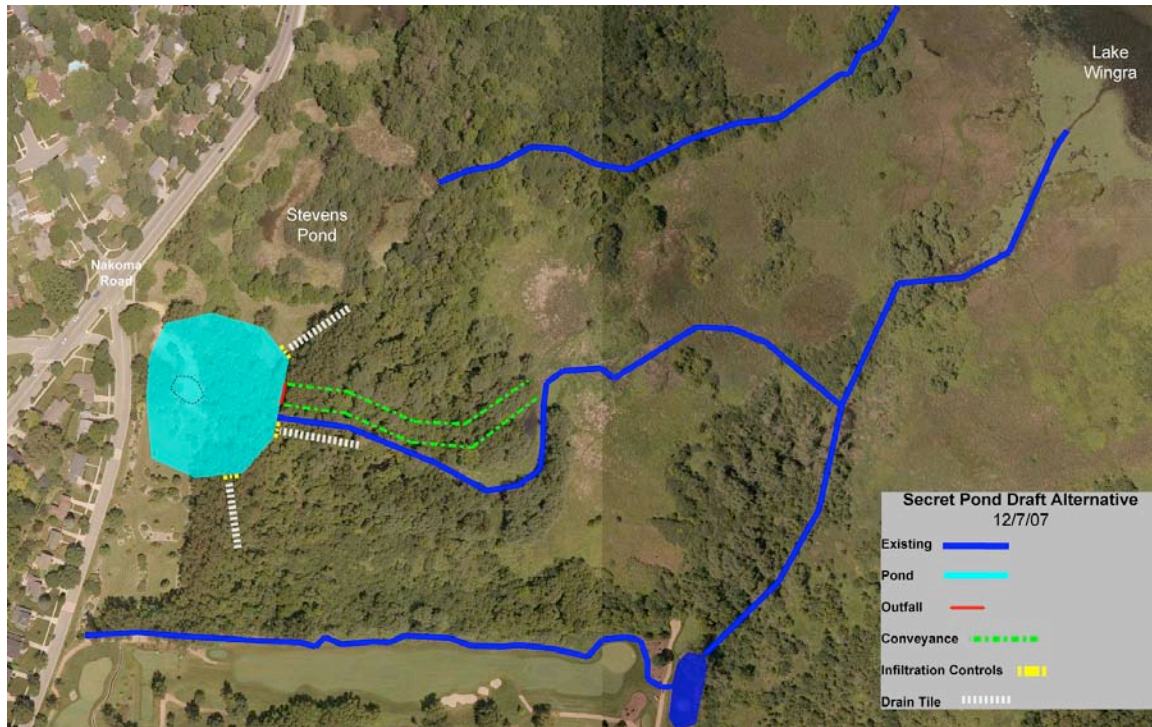
Figure 9: Recently proposed (12/2007) single channel design for Secret Pond. Created with input from Joy Zedler, Kevin McSweeney, Dave Liebl and Ken Potter.
